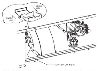
FIG. 58 Adjusting Air Shutter 990,000 - 2,070,000 Btu/hr Models
